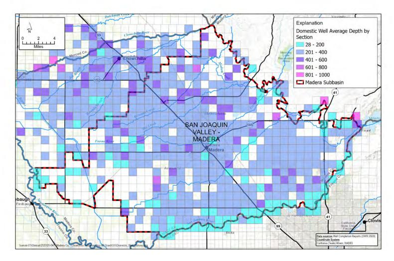
Figure 7b. Domestic Wells in Madera Subbasin with Average Depth by Township/Range/Section.
