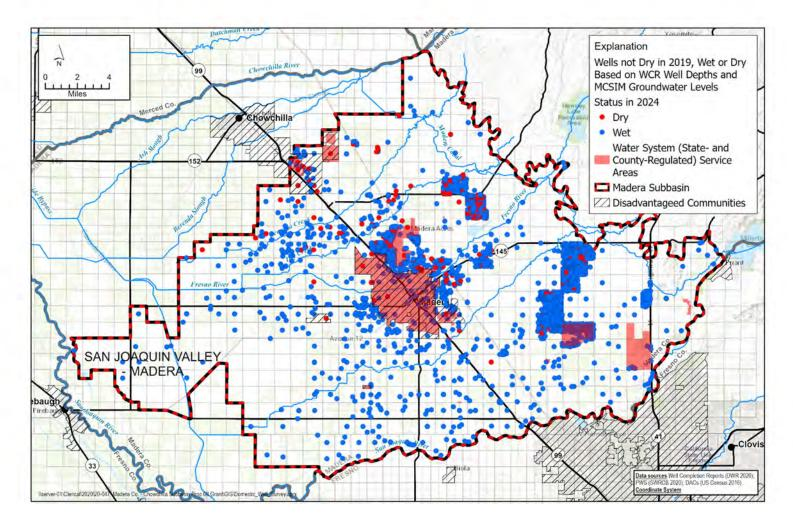
Figure 13b: Status of Wells in 2024 - Based on WCR Well Depths and Locations Compared to MCSIM Groundwater Depths.
