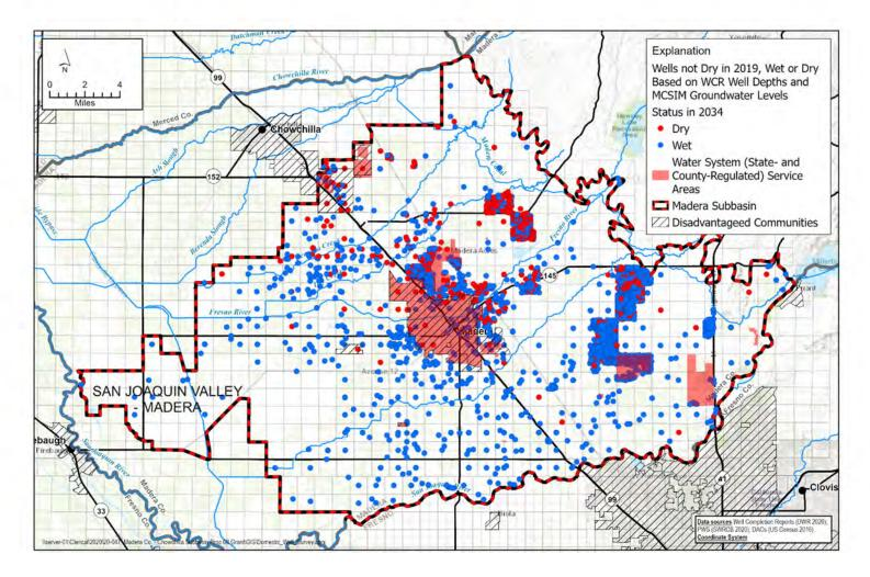
Figure 13d: Status of Wells in 2034 - Based on WCR Well Depths and Locations Compared to MCSIM Groundwater Depths.
