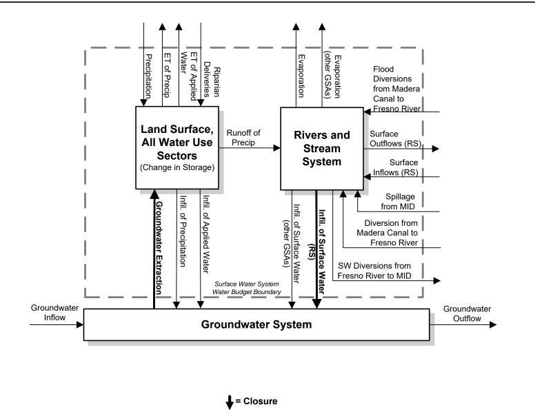
Figure A2.F.b-2. Madera County GSA Water Budget Structure.
