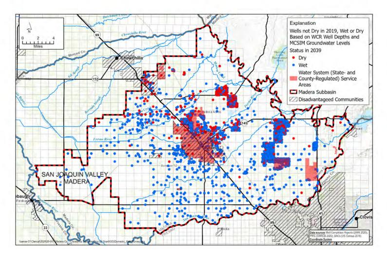
Figure 13e: Status of Wells in 2039 - Based on WCR Well Depths and Locations Compared to MCSIM Groundwater Depths.
