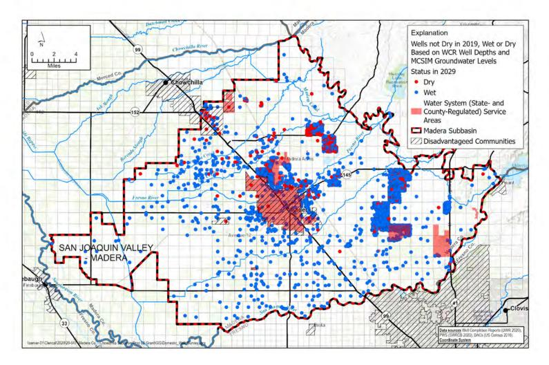
Figure 13c: Status of Wells in 2029 - Based on WCR Well Depths and Locations Compared to MCSIM Groundwater Depths.
