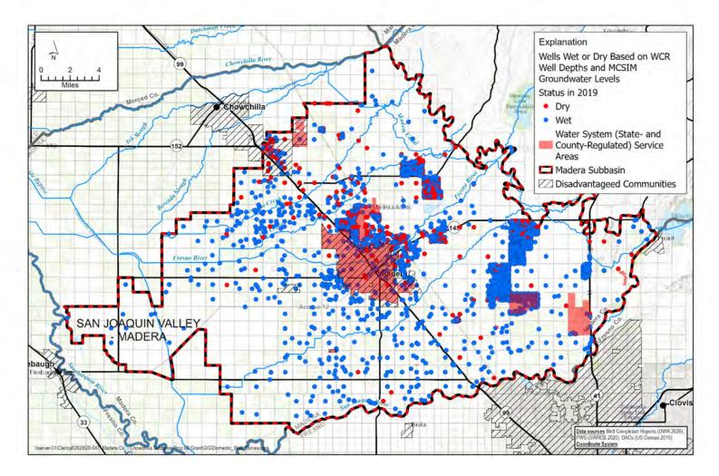
Figure 13a: Status of domestic wells in 2019 - Based on WCR well depths and locations compared to MCSIM groundwater depths.
