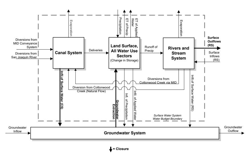
Figure A2.F.e-2. Gravelly Ford Water District GSA Water Budget Structure
