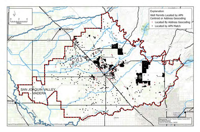
Figure 2a: Permit locations and geolocation method in Madera Subbasin.
