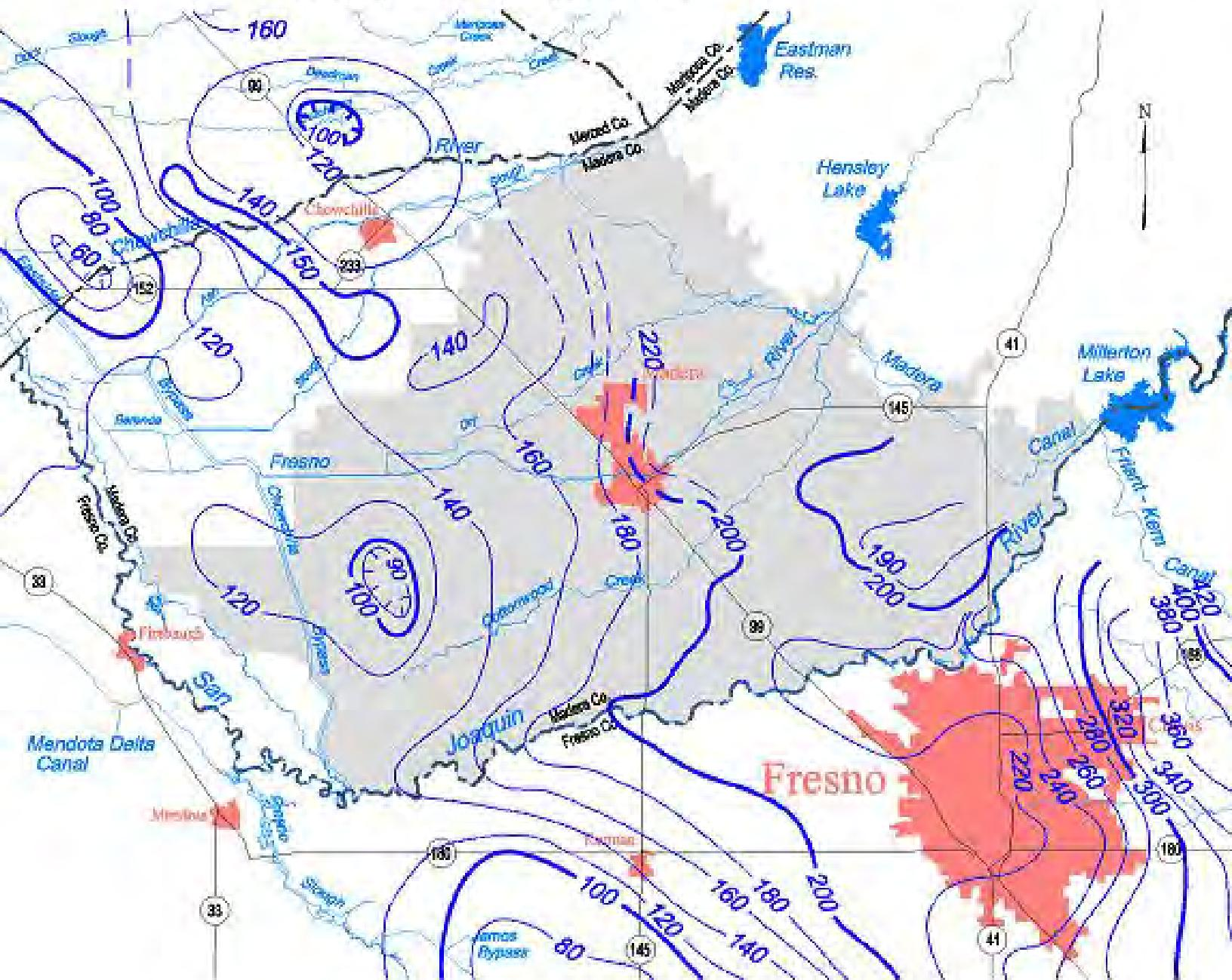
Contours are dashed where inferred. Contour interval is 10 and 20 feet.
