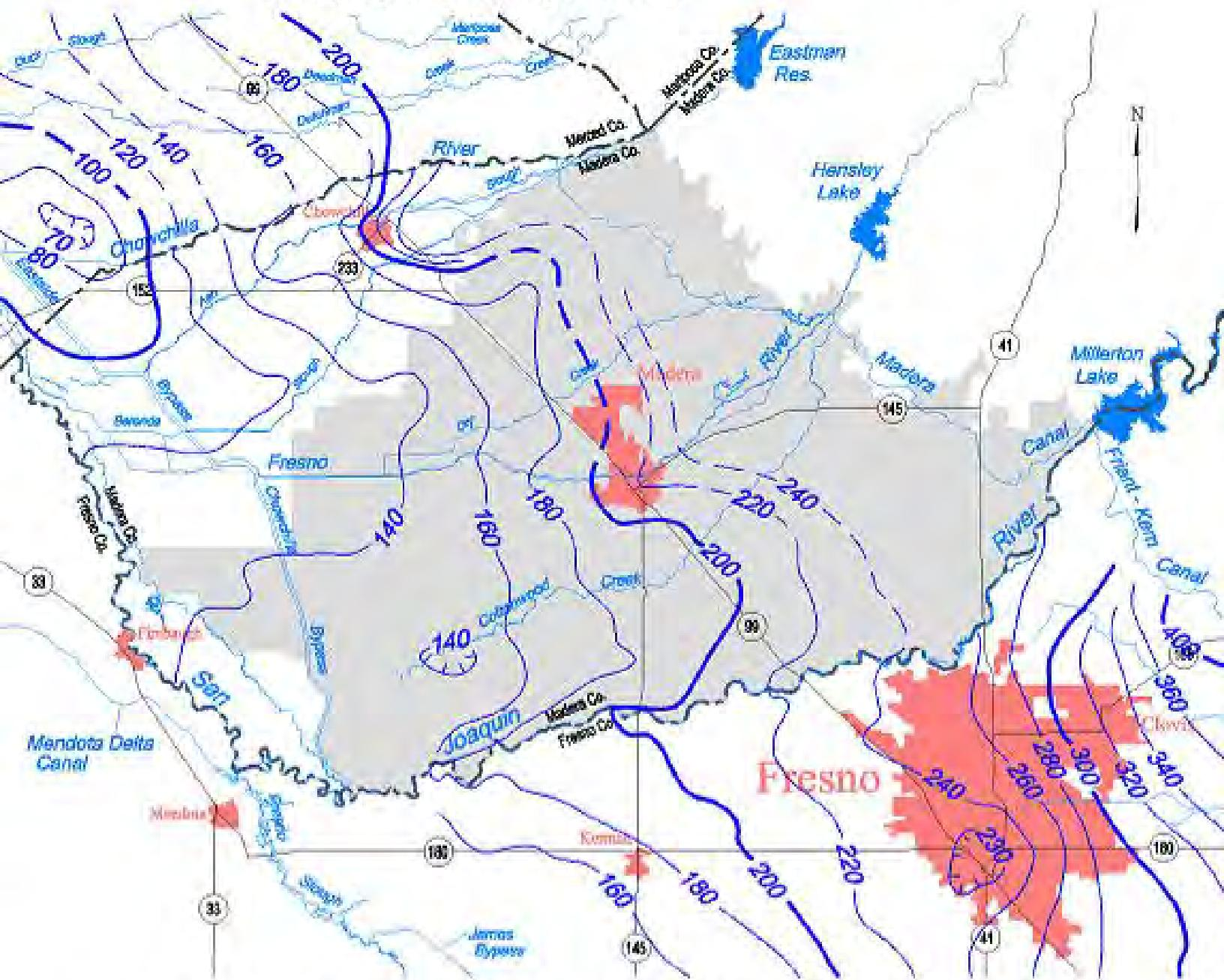
Contours are dashed where inferred. Contour interval is 10, 20 and 40 feet.
