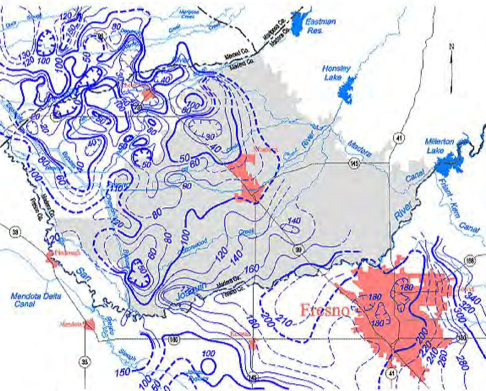
Contours are dashed where inferred. Contour interval is 10, 20 and 50 feet.
