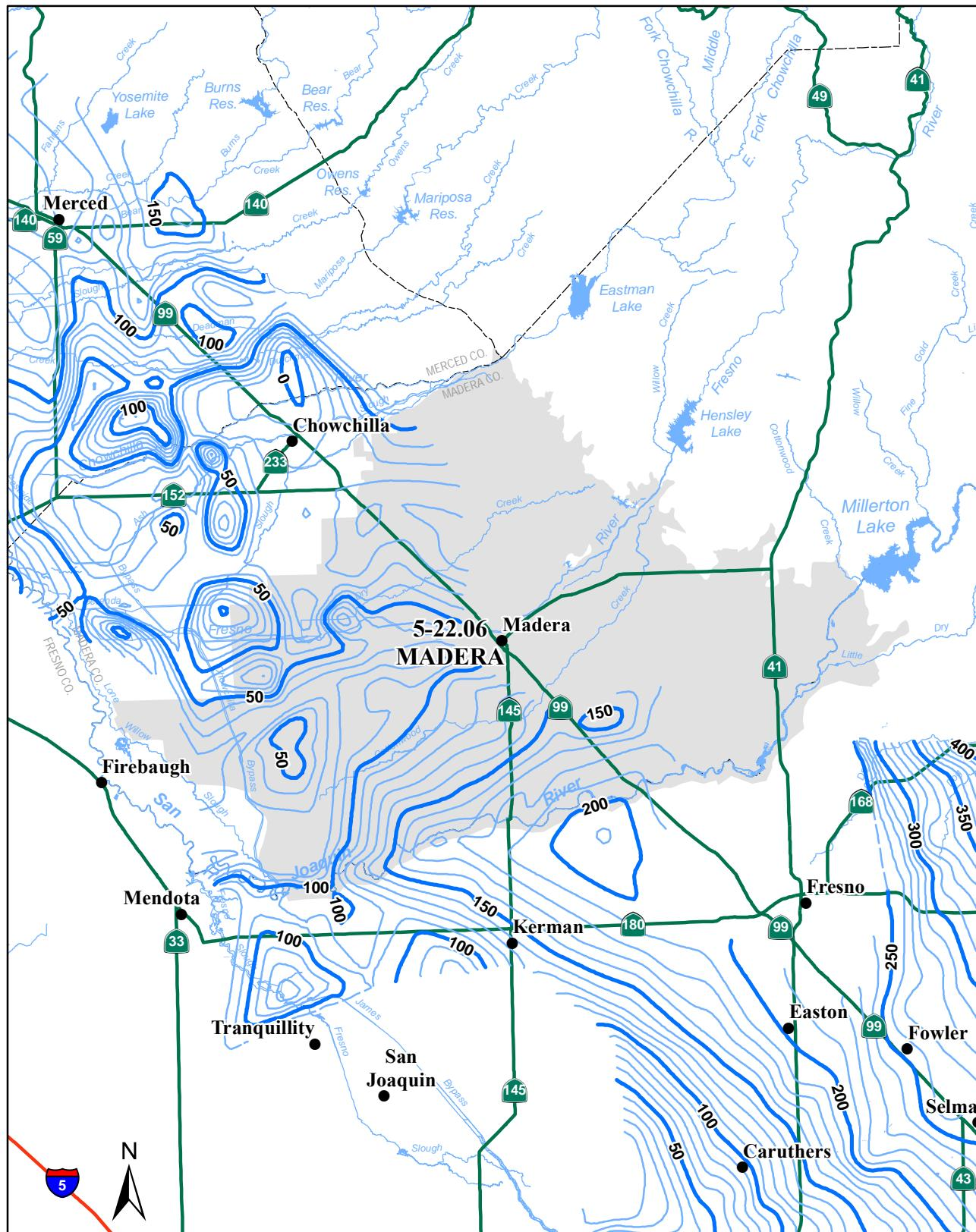
Lines of equal elevation of groundwater in feet above mean sea level.
