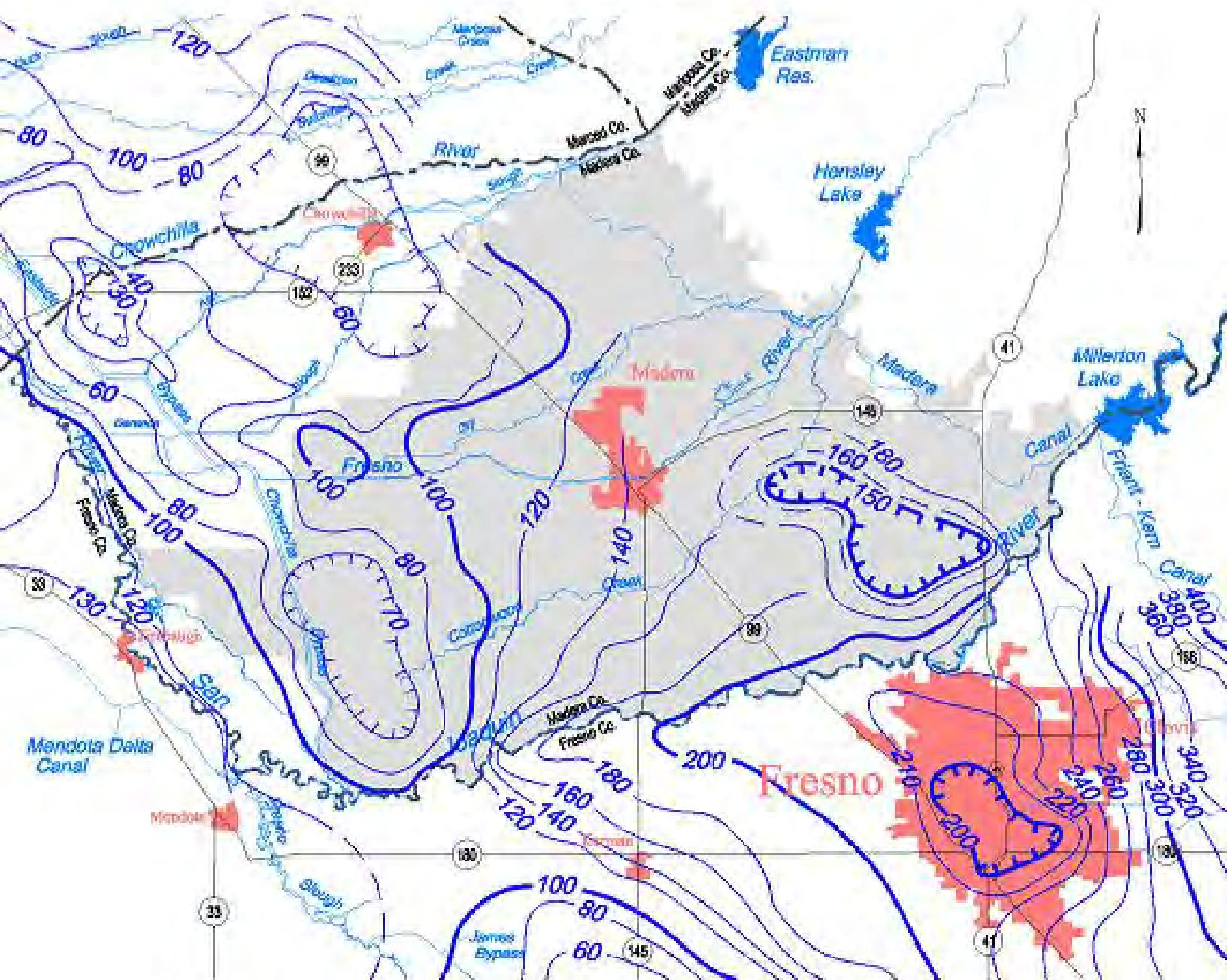
Contours are dashed where inferred. Contour interval is 10 and 20 feet.
